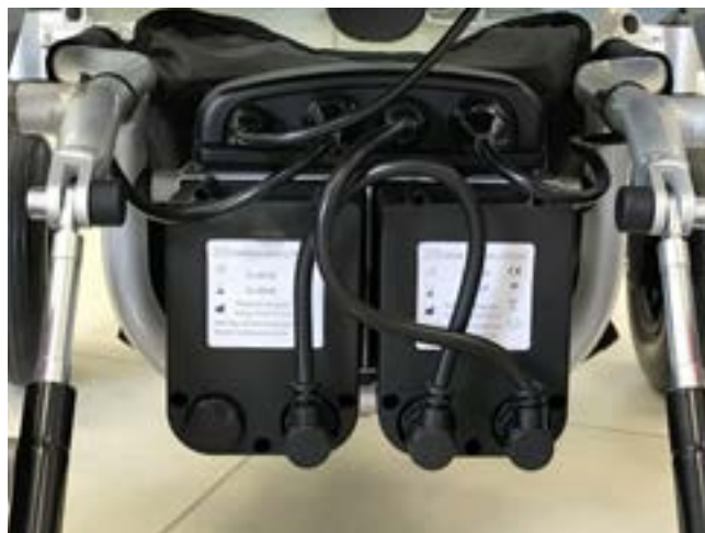
A06/L & S1 with 2 batteries
