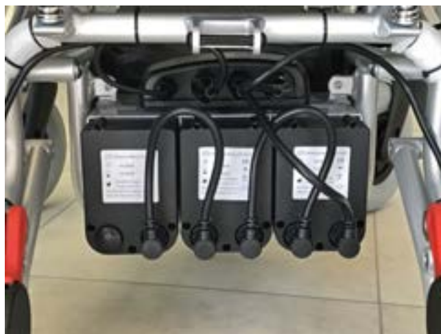
A08/L & DE08L with 3 batteries
